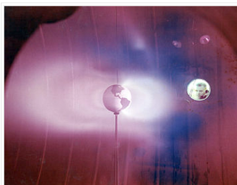
Simulated Van Allen Belts generated by a plasma thruster in tank #5 Electric Propulsion Laboratory at the then-called Lewis Research Center, Cleveland Ohio,
